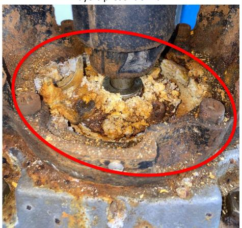
Treated pump, the image shows significant improvement in reducing scale layers as shown in the image almost all white scale layers are being removed.
