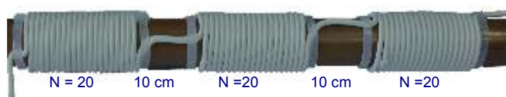
Three coils in series. Induction will be less. However treatment time will be much longer.
