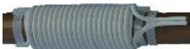
Coil with two layers on top of each other. Twenty windings each. This doubles the induction.
