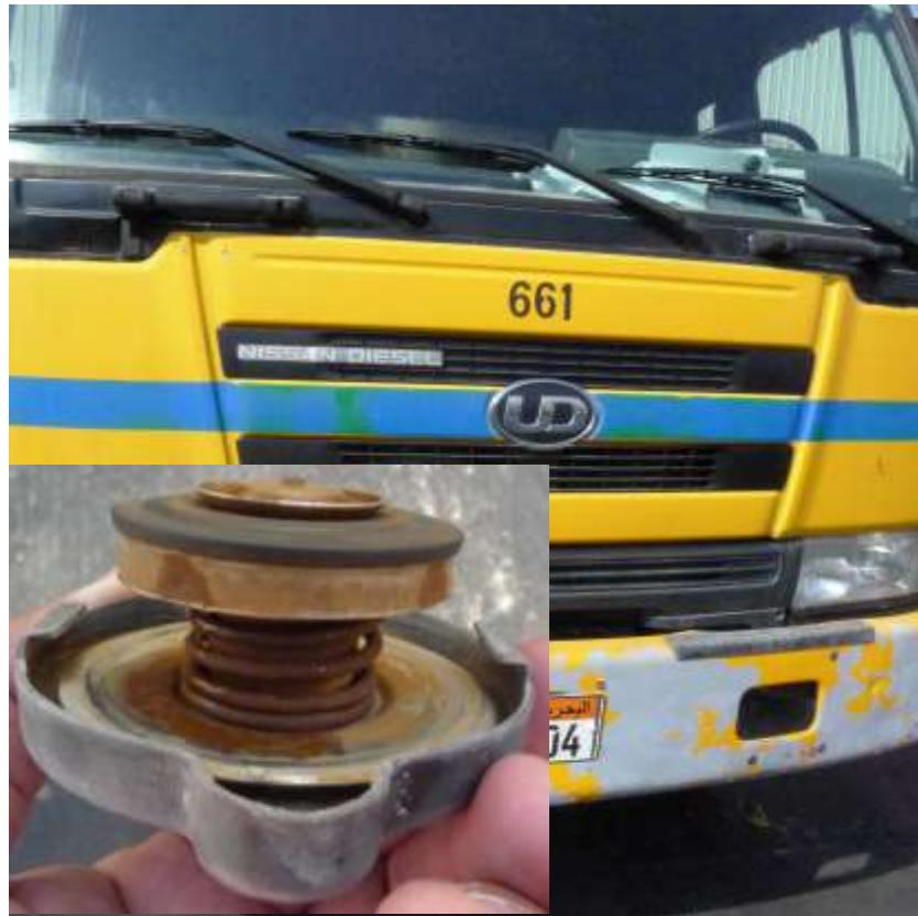
Truck #642 **with SW TRP system for 60 days:** radiator cap and circulating water
