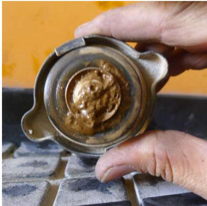
November 10, 2016- 60 days after installation. Actual status of the radiator cap directly after taking it off from the reservoir. (**Cleaner**)
