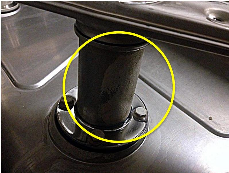
6<sup>th</sup> Nov 2016, the scaling patch is being removed and is not visible anymore and plus it is much shinier and smoother than the previous one.
