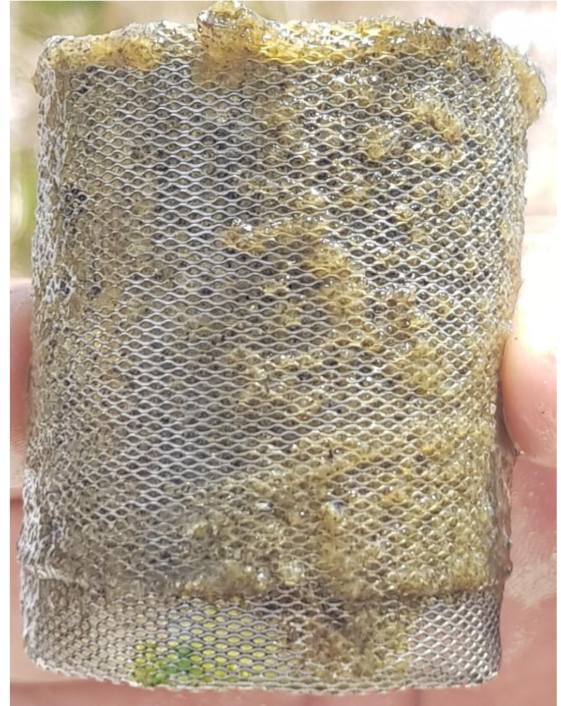
After Installation, 27 th June 2019 Less and Dull yellowish microorganism on some parts of strainer
