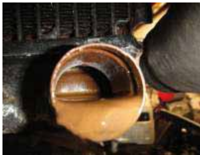
Rusty radiator sludge
