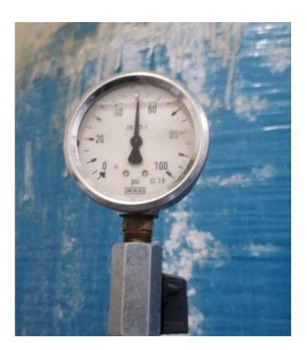
After treatment (week 6), the image clearly shows that the pressure in guage has dropped due to melting of scaling in the pipeline
