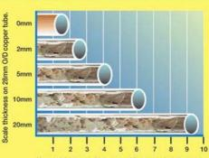
Hours to heat one days uage of hot water in a domestic indirect cylinder.
